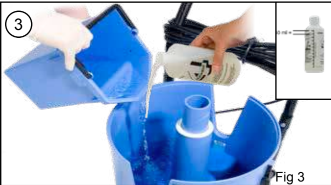
Fill the NuChem / water tank, up to the full level mark, avoid pouring fluids into the central tube as this leads directly to the vacuum motor (Fig 3).
